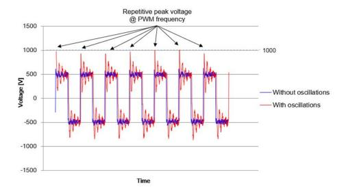
Figure 5.2.1.4 Voltage oscillation schematic (750 V\_DC controller)
