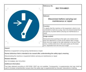
Figure 7.1.4 Example of a warning sign
