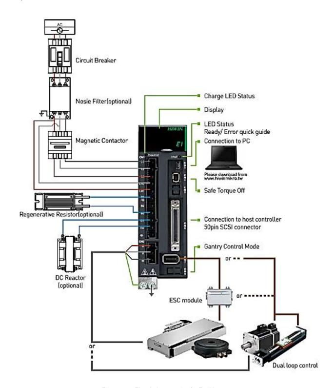
Figure 5.2.1 Electrical connection for E1 drive
