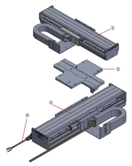
Figure 3.2.1 Main components of LMSSA2X
