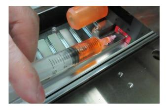
Figure 7.1.4.1.2 MGN Block grease maintenance kit
