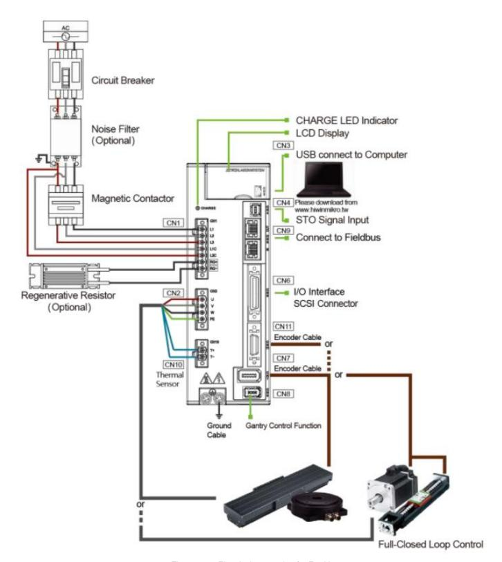
Figure 5.2.2 Electrical connection for E2 drive
