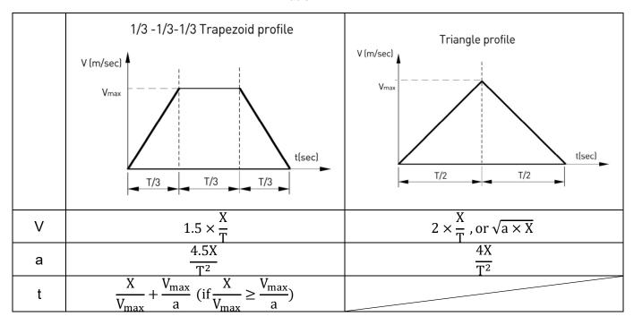
The acceleration required in the first motion velocity profile is bigger than that in the second motion velocity profile; therefore, the required motor size is bigger. When choosing second motion velocity profile, the chosen motor size is smaller, however, we need to verify the DC bus of driver is bigger enough, due to the higher velocity  $(V_{\rm max})$ .
