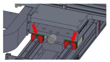
Figure 7.1.4.1.1 Grease nipples on linear guideways
