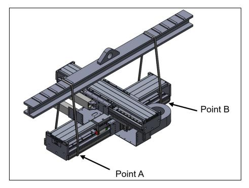
Figure 4.2.1 Hoisting and transporting
