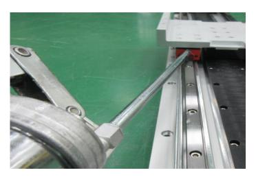
圖. 7.1.4.1.3 QH Block grease maintenance kit
