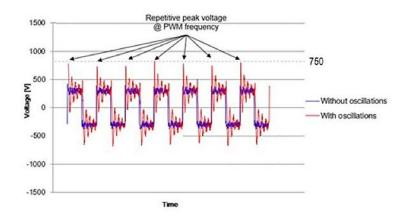
Figure 5.2.1.3 Voltage oscillation schematic (325 V\_DC controller)
