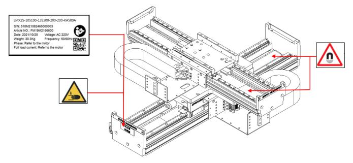
Figure 2.8.1 Warning symbols and plate – here for LMSSA2X
