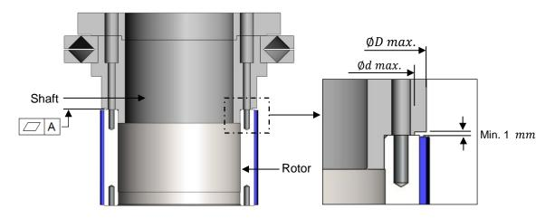
Figure 4.6 Rotor mounting interface (TMRW/TM-2)
