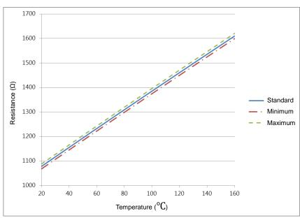
Figure 4.25 Relationship between resistance and temperature (Pt1000)
