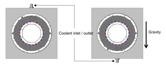
Figure 4.4 Coolant inlet / outlet position when mounted vertically
