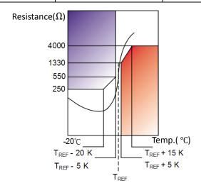
Figure 4.26 Relationship between PTC temperature and resistance
