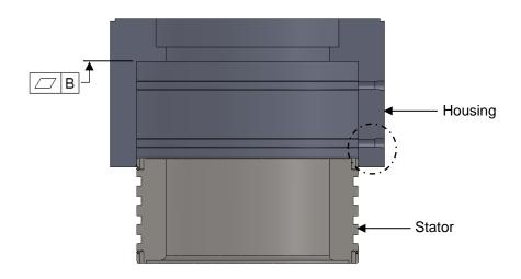
Figure 4.8 Stator mounting interface
