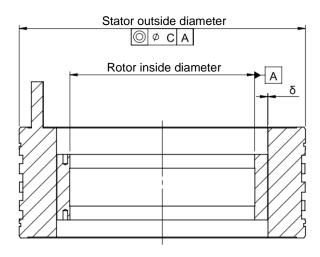
Figure 4.10 Air gap and assembly concentricity diagram
