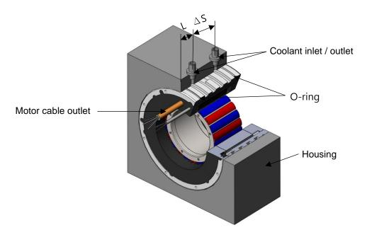
Figure 4.1 Basic structure of HIWIN torque motor
