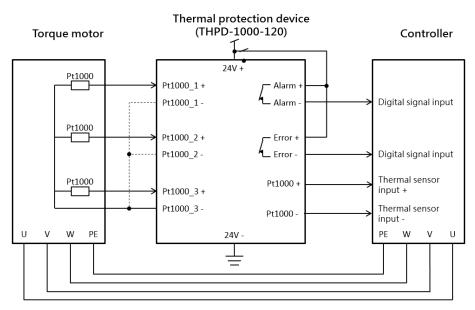
Figure 5.2 Pt1000 wiring diagram
