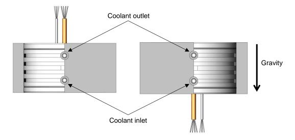
Figure 4.3 Coolant inlet / outlet position when mounted horizontally
