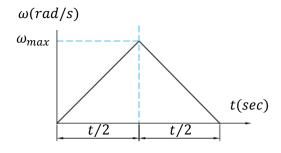
$$\omega_{max} = 2 \times \frac{\varphi}{t} \stackrel{\text{def}}{=} \omega_{max} = \sqrt{\alpha \times \varphi}$$
