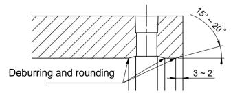
Figure 4.9 Housing mounting interface
