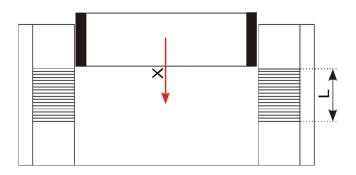
Figure 4.12 Axial offset of the stator and rotor
