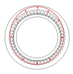
Figure 4.11 Concentricity of stator and rotor is offset
