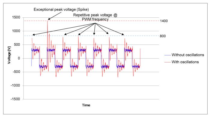
Figure 3.2 Voltage oscillation schematic (600/750  $V_{DC}$  controller)
