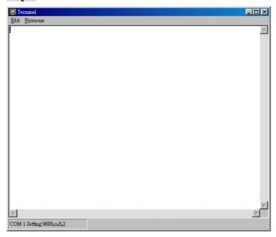
**Step2:** Keep pressing "Back Space" on keyboard, and turn on power of LMDX driver, then it enters "Monitor" mode. Now the orange and red LED will blink twice to show that it is under "Monitor" mode. Now terminal may look like this.
