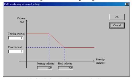
Fig. 30 Field weakening advanced settings
