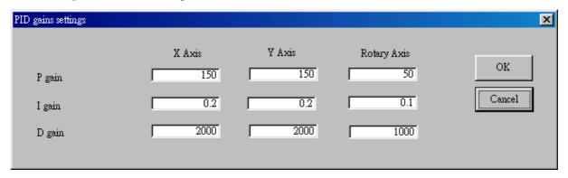
Fig. 23 PID gains
