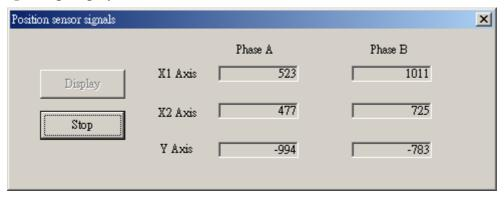
Fig. 38 Display status for sensor
