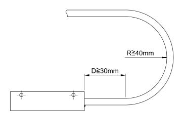
Figure 5.1.2.1 Specifications of outlet and bending radius for readhead
