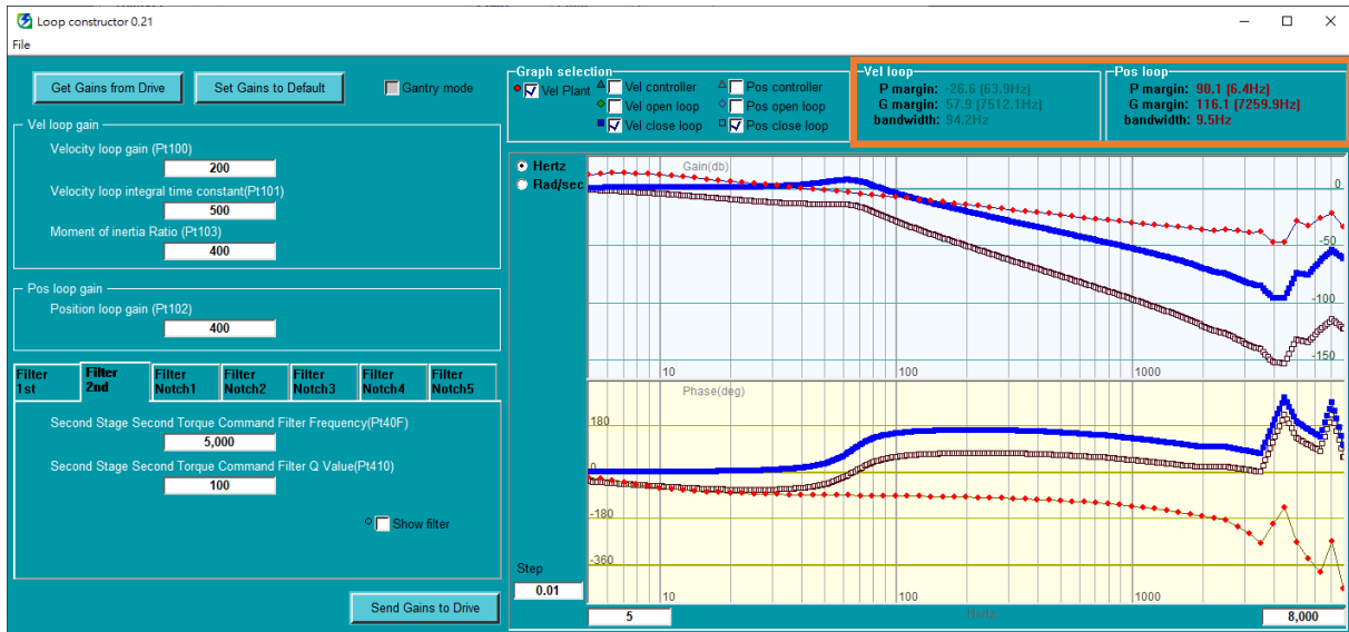
Figure 6.3.1.3.2 P margin, G margin and bandwidth
