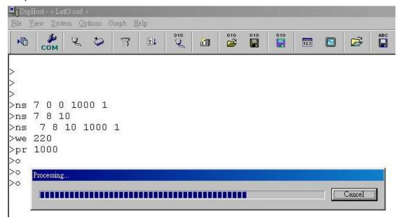
Step 2: After downloading data with 'O' command, it is necessary to set array parameters (F7-key), the picture will show like below.
