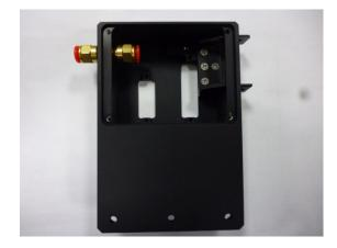
Step 8: Put motor cable connector pass through the connector-mount-seat; mount the connector by the copper roller (just fasten the copper roller; don't break the roller).
