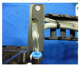
Step 6: One-by-one assemble the square chain pieces from the chain mount-seat until 5~6 pieces are left.
