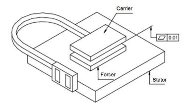
b. Same case, the flatness of stator-seat surface should be less than 0.01mm/300mm; otherwise, stator may deform.
