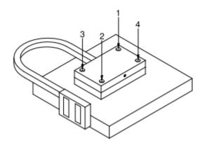
d. Do not put any strong magnetic substance around the forcer that would affect the normal moving of forcer.
