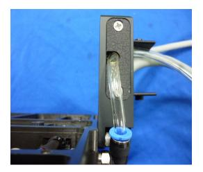
Step 5: After the square chain and flange (male end) are connected, fix the tubes and square chain by cable-tie.
