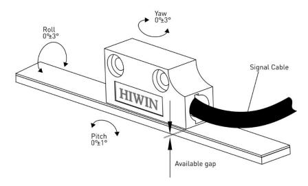
Figure 5.1.3.1 Installation specifications for E type read head
